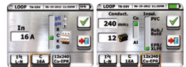
Setting of MCB/fuse type and rated current
