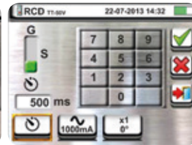
Setting of RCD delayed time
