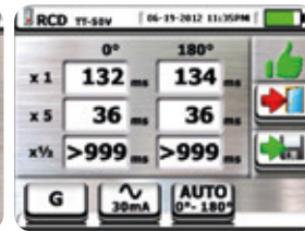
AUTO test result on RCD
