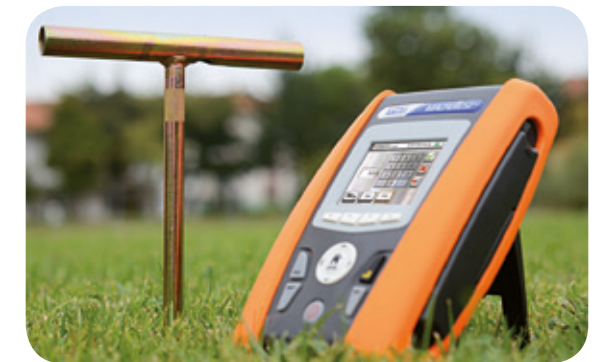
Earth resistance measurement by Volt-ampere method
