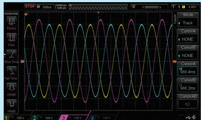
Three Phase Unbalance Voltage Test Captured
