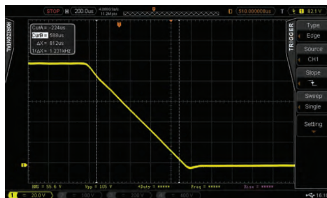
DC Voltage Ramp Down @ 100Vdc/ms programmed slew rate into 100Ω resistive load captured
